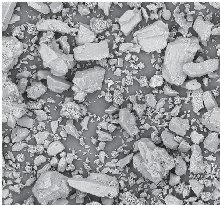
Fig. 2: SEM picture of a not fully reacted Magnesium Taurate (Photo®: Dr. Paul Lohmann GmbH & Co. KGaA)
